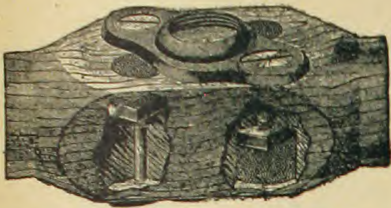
SECTION OF CROSS-ARM, SHOWING METHOD OF BOLTING THE FIT- TINGS (No screws to work loose in the wood.)
